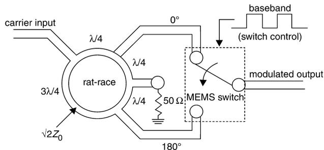
Fig. 1 Diagram of proposed BPSK modulator
