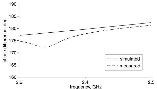
Fig. 2 Simulated and measured BPSK carrier output phase difference
