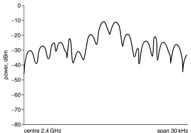
Fig. 3 Spectrum of BPSK modulator with carrier frequency of 2.4 GHz and 1 kHz square-wave modulating signal
