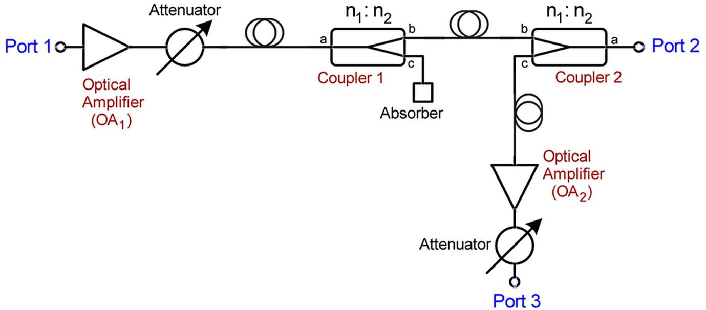
Fig. 2. Schematic diagram of the optical quasi-circulator.
