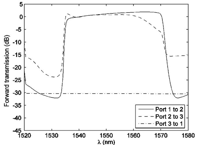
Fig. 3. Measured forward response of the quasi-circulator.
