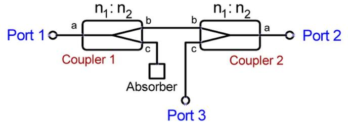
Fig. 1. Two identical back-to-back optical couplers.
