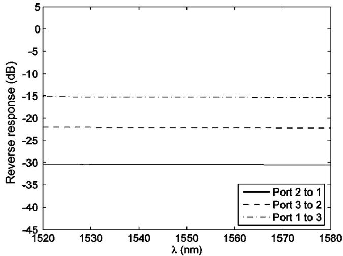
Fig. 4. Measured isolation between various ports of the quasi-circulator.
