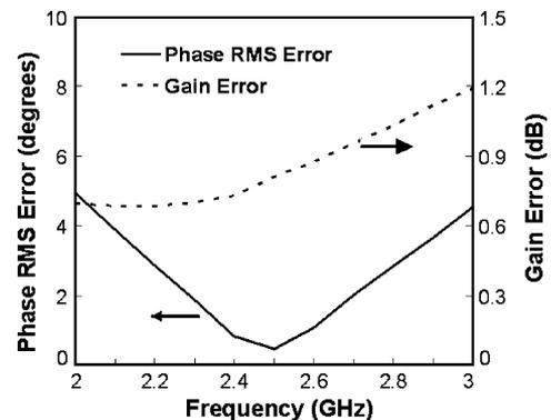
Fig. 10. RMS phase error and gain error versus frequency.
