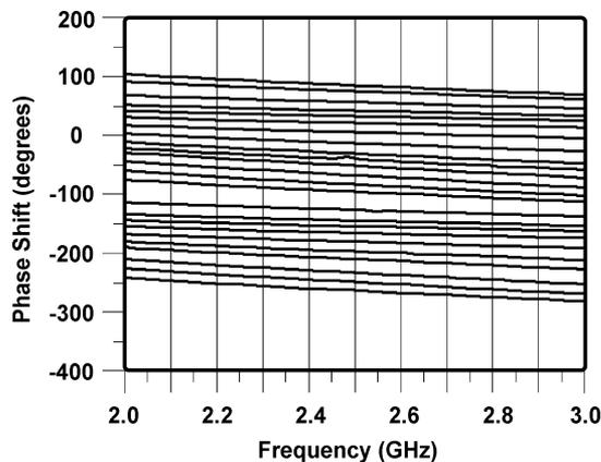
Fig. 7. Measured phase shift versus frequency and control voltage,  $V_{C7}$ .
