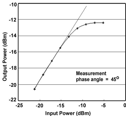
Fig. 12. Measured RF power performance (data taken at 45° phase shift).
