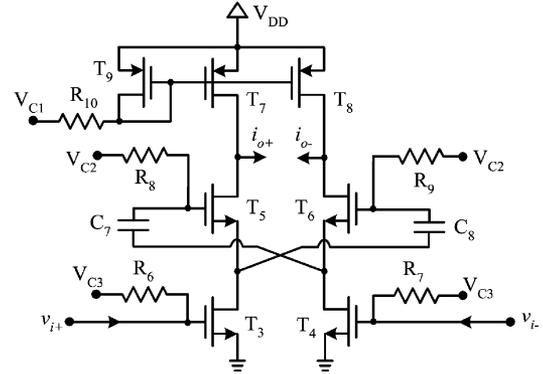
Fig. 4. OTA circuit using a feedforward-regulated topology.
