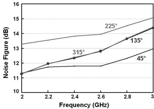
Fig. 11. Measured noise figure (NF) at various phase angles.
