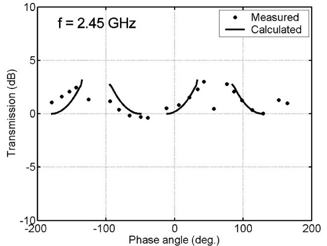
Fig. 8. Transmission coefficient ( $S_{21}$ ) versus phase angle,  $\phi_{out}$ .
