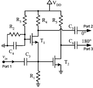
Fig. 2. Active balun circuit.
