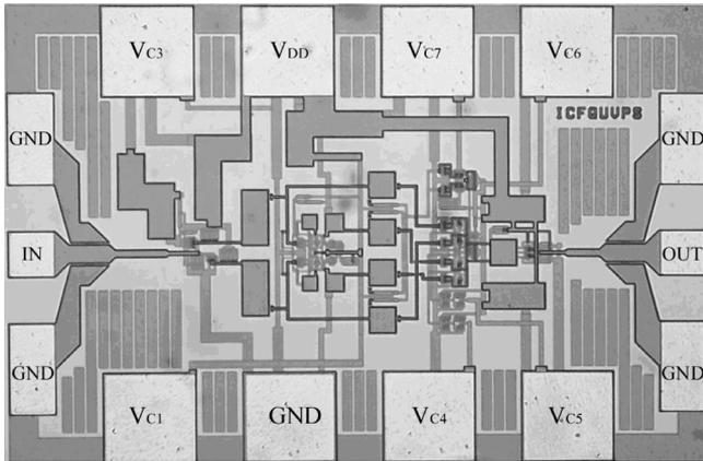
Fig. 6. Microphotograph of the fabricated phase shifter.
