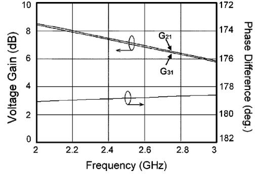
Fig. 3. Balun amplitude and phase response (simulated).
