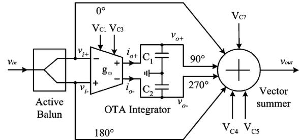
Fig. 1. Proposed 360° vector-sum phase shifter circuit.
