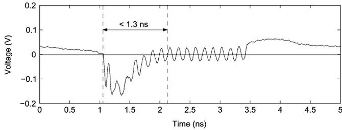
Fig. 15. Measured time-domain output at 200 MHz (one clock period).
