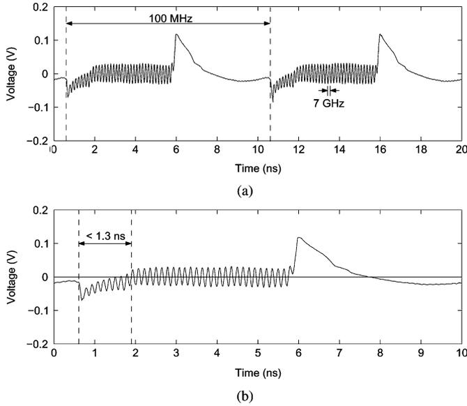
Fig. 14. Measured time-domain output at 100 MHz. (a) Two clock periods. (b) One clock period.
