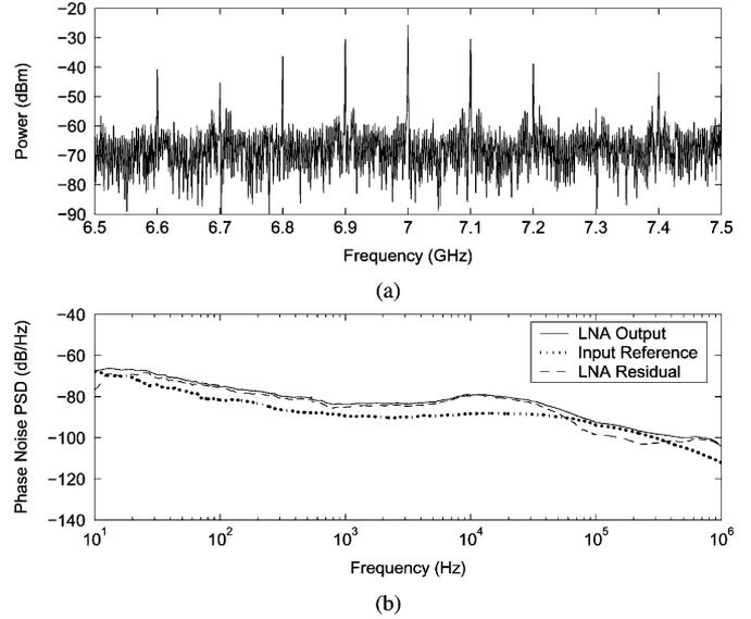
Fig. 16. Measured LNA output. (a) Power spectrum. (b) Phase noise.
