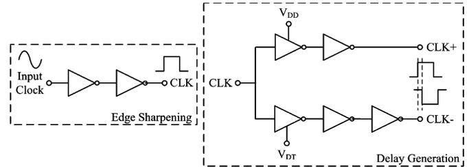
Fig. 10. Clock edge sharpening and delay generation circuits.
