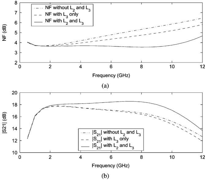
Fig. 4. Simulated LNA NF and gain  $|S_{21}|$  with and without inductors  $L_2$  and  $L_3$ .
