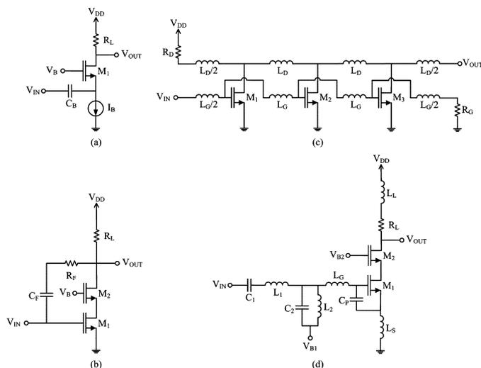
Fig. 1. Common wideband LNA topologies. (a) Common gate. (b) Shunt resistive feedback. (c) Distributed. (d) Passive input matching.
