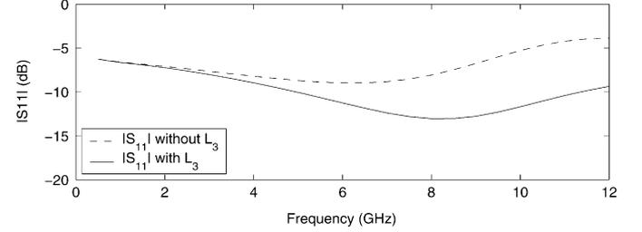
Fig. 6. Simulated LNA input reflection coefficient  $|S_{11}|$  with and without inductor  $L_3$ .
