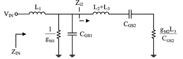
Fig. 5. Small-signal model of the input matching network.
