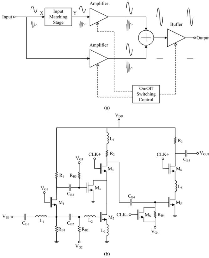
Fig. 2. Block diagram and circuit schematic of the proposed LNA.
