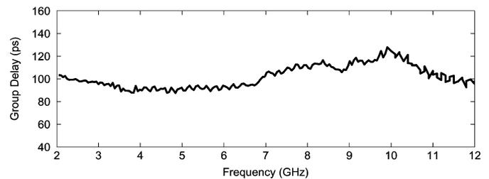
Fig. 13. Measured LNA group delay from 2 to 12 GHz.
