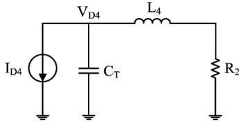
Fig. 7. Two-pole shunt inductive peaking network.
