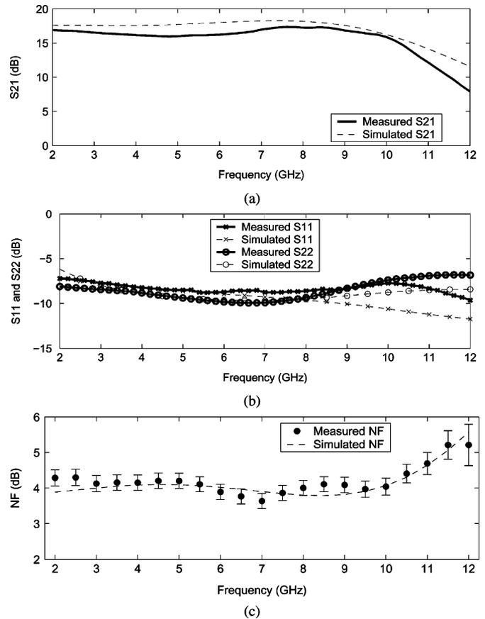
Fig. 12. (a) and (b) Measured LNA two-port  $S$ -parameters and (c) NF.
