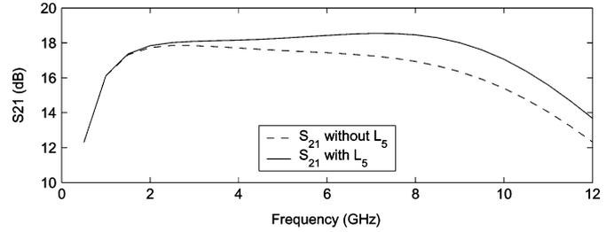
Fig. 9. Simulated LNA gain  $|S_{21}|$  with and without inductor  $L_5$ .
