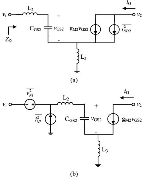
Fig. 3. Small-signal model of  $M_2$  with  $L_2$  and  $L_3$ . (a) Output drain-source noise current  $i_{ND2}^2$  and (b) input-referred noise voltage  $v_{NI}^2$  and current  $i_{NI}^2$ .
