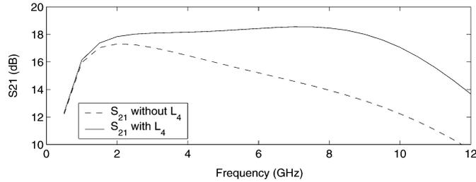
Fig. 8. Simulated LNA gain  $|S_{21}|$  with and without inductor  $L_4$ .
