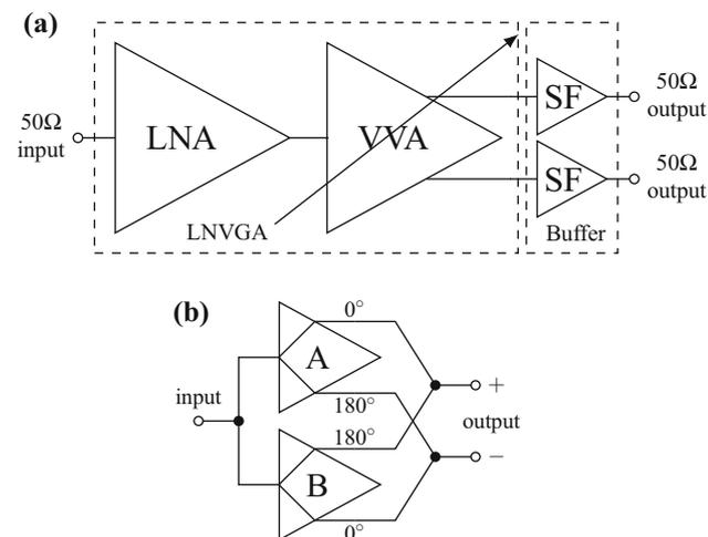
**Fig. 1** Block diagram of the LNVGA with the measurement buffer (a). The VVA composed of two baluns (b)
