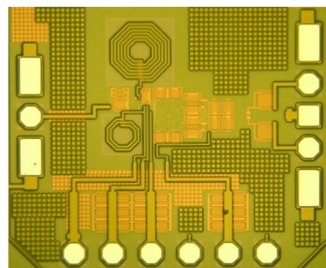
**Fig. 5** The photograph of the LNVGA chip
