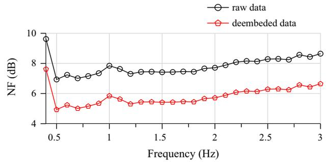
**Fig. 8** Measured NF at maximum gain
