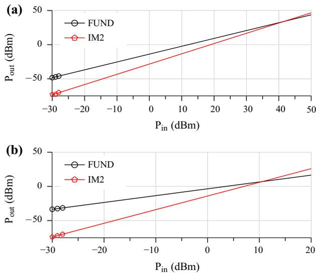
**Fig. 10** Best case IIP2 at  $V_{crit} = 0.7$  V (a) and worst case IIP2 at  $V_{crit} = 0$  V (b)
