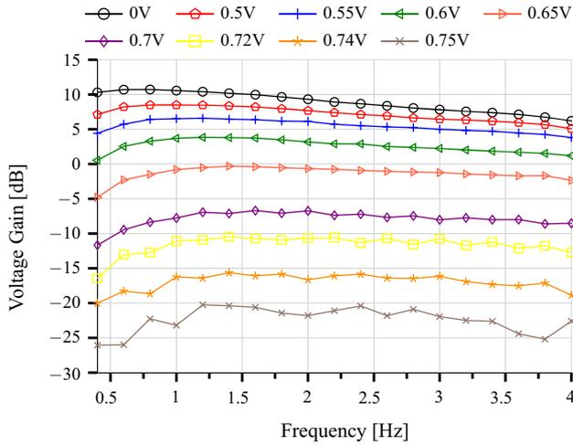
**Fig. 6** Measured voltage gain and gain control range
