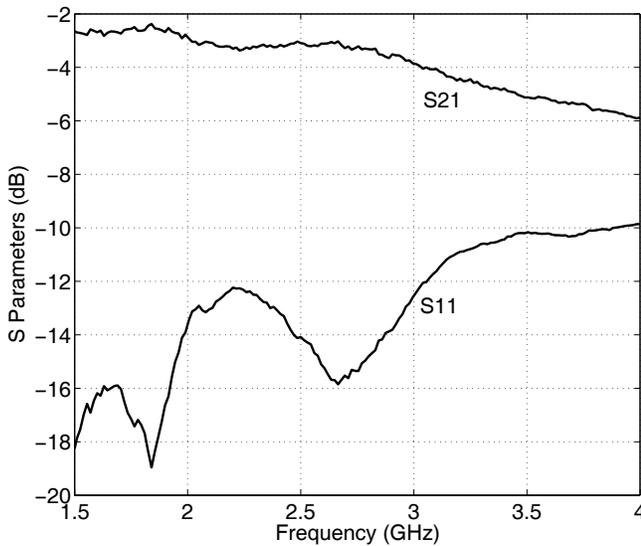
Figure 3. Measured input return loss and insertion loss
