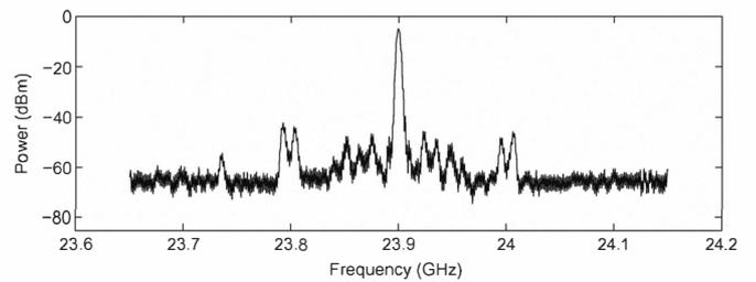
Fig. 5. Measured free-running output spectrum over a span of 500 MHz.
