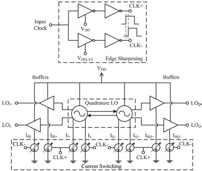
Fig. 1. Circuit diagram of quadrature pulsed oscillator.
