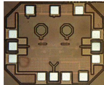
Fig. 4. Photograph of quadrature pulsed oscillator IC.
