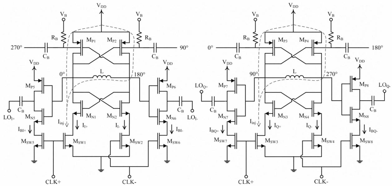
Fig. 2. Circuit schematic of quadrature LC oscillators and buffers.
