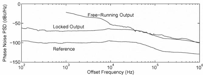
Fig. 7. Measured phase noise of pulsed output at 24 GHz.
