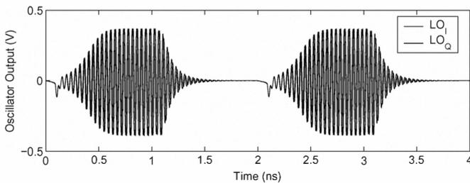
Fig. 3. Simulated pulsed oscillator waveforms.
