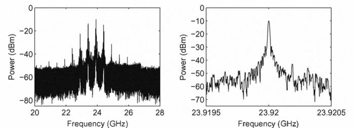
Fig. 6. Measured pulsed output spectrum over an 8 GHz span (left) and a 1 MHz span (right).
