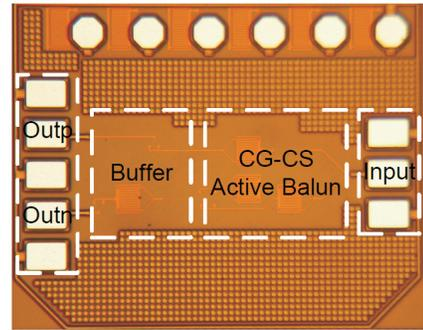
Fig. 5. Chip microphotograph.
