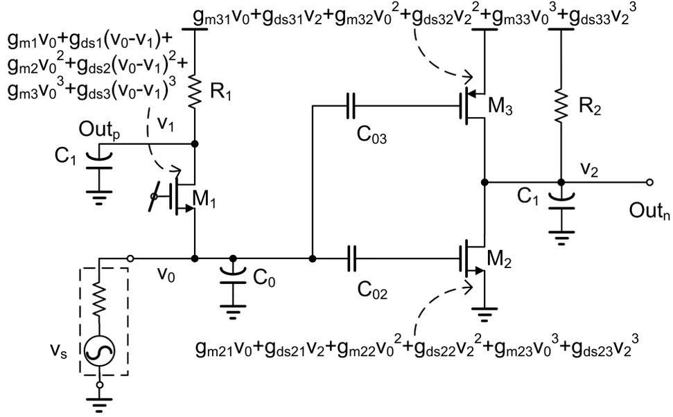
Fig. 1. Circuit schematic of the wideband, low-voltage, active balun and amplifier circuit.
