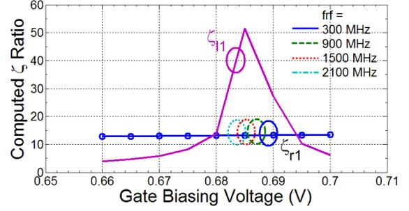
Fig. 2. Computed  $\zeta$  ratio of the CG-CS active balun based on the analysis.
