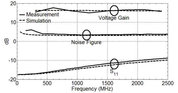
Fig. 4. Measured and simulated  $S_{11}$ , noise figure, and the voltage gain vs. RF frequency.
