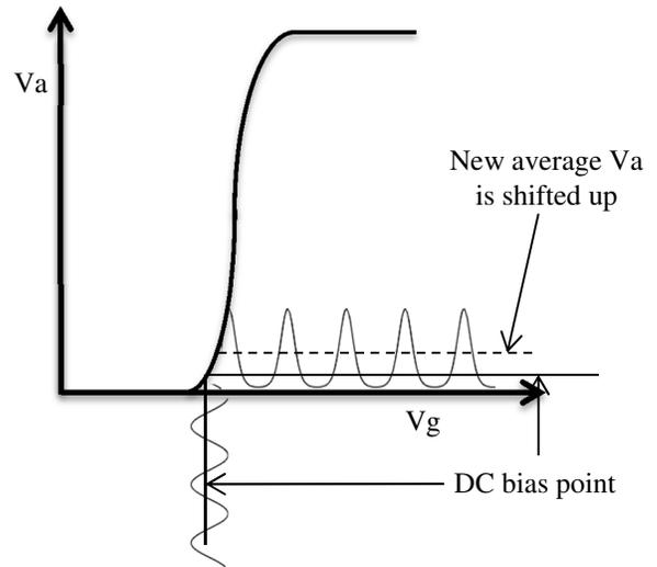
**Fig 3. RF amplifier biased in its nonlinear region for envelope detection.**
