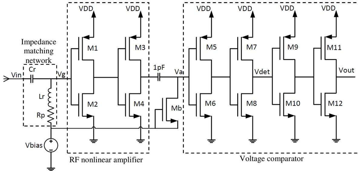
**Fig 2. Overall Circuit architecture.**
