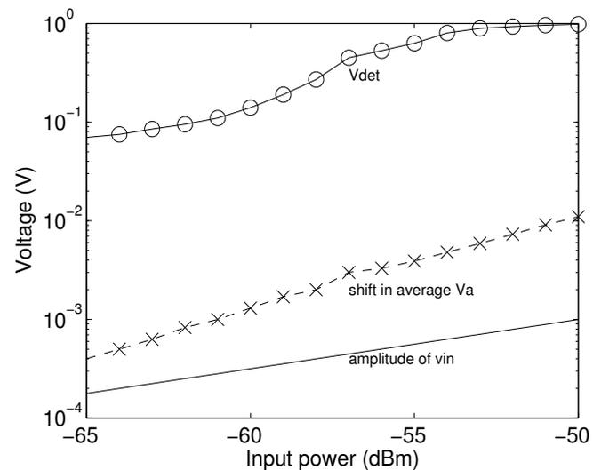
Fig 5:  $V_{in}$ , shift in  $V_a$ , and detection voltage all plotted against input power.
