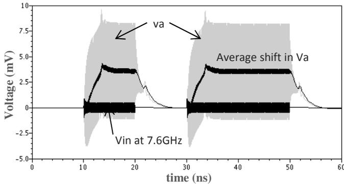
Fig 8. Waveforms for Va in response to -55dBm input power.
