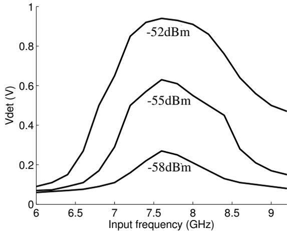
Figure 7: Dependence of detection voltage on frequency of input signal for different input powers.
