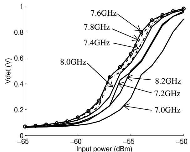
Fig 6: Dependence of detection voltage on power of input signal for different input frequencies.
