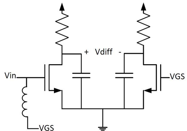
Fig 1. Typical envelope detector for low power signals.
