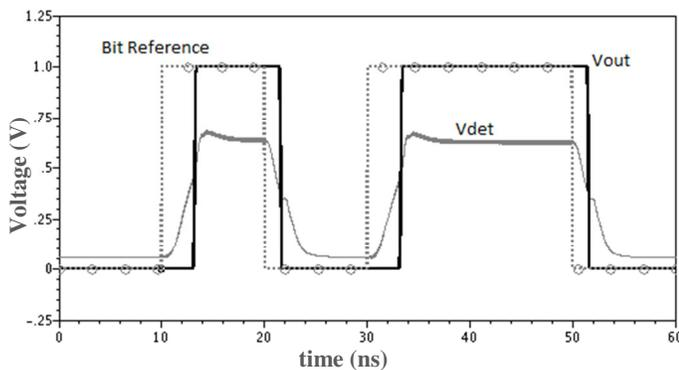
Fig 9: Digital level waveforms in response to -55dBm input power.
