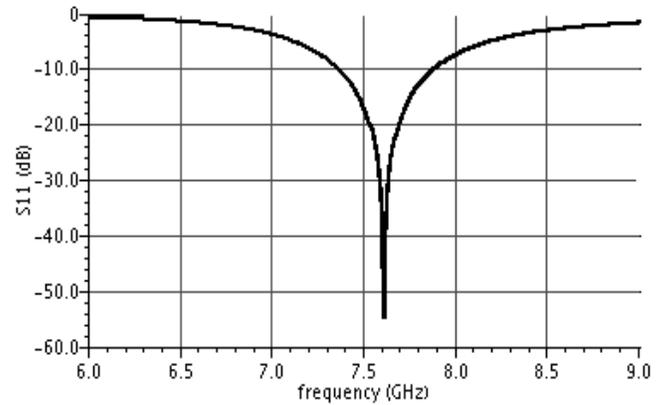
Fig 4. Reflection coefficient at input of power detector.
