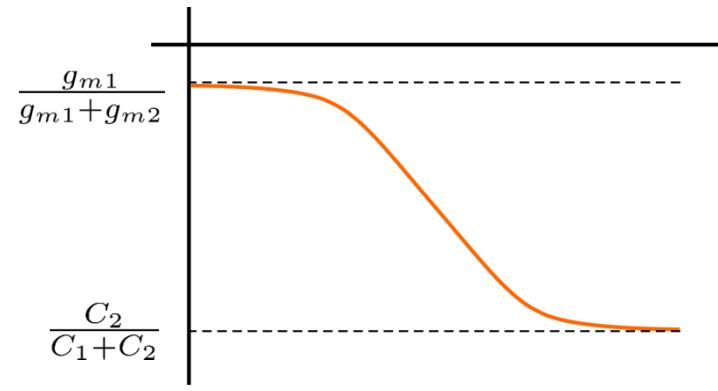
$$\frac{v_{out}}{v_{in}} = \frac{g_{m1} + sC_2}{s(C_1 + C_2) + g_{m1} + g_{m2}}$$
