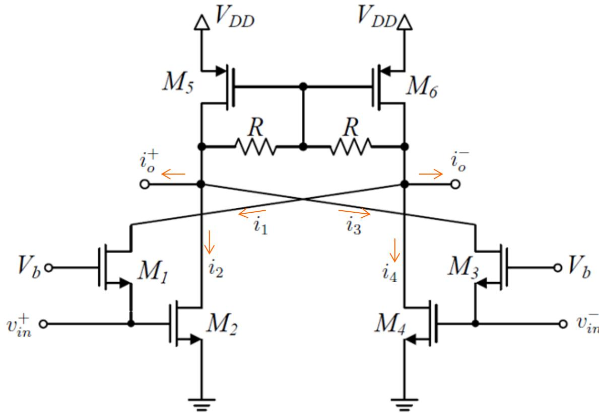
$$i_o^+ = i_2 + i_3 = g_{m2}v_{in}^+ - g_{m3}v_{in}^-$$
